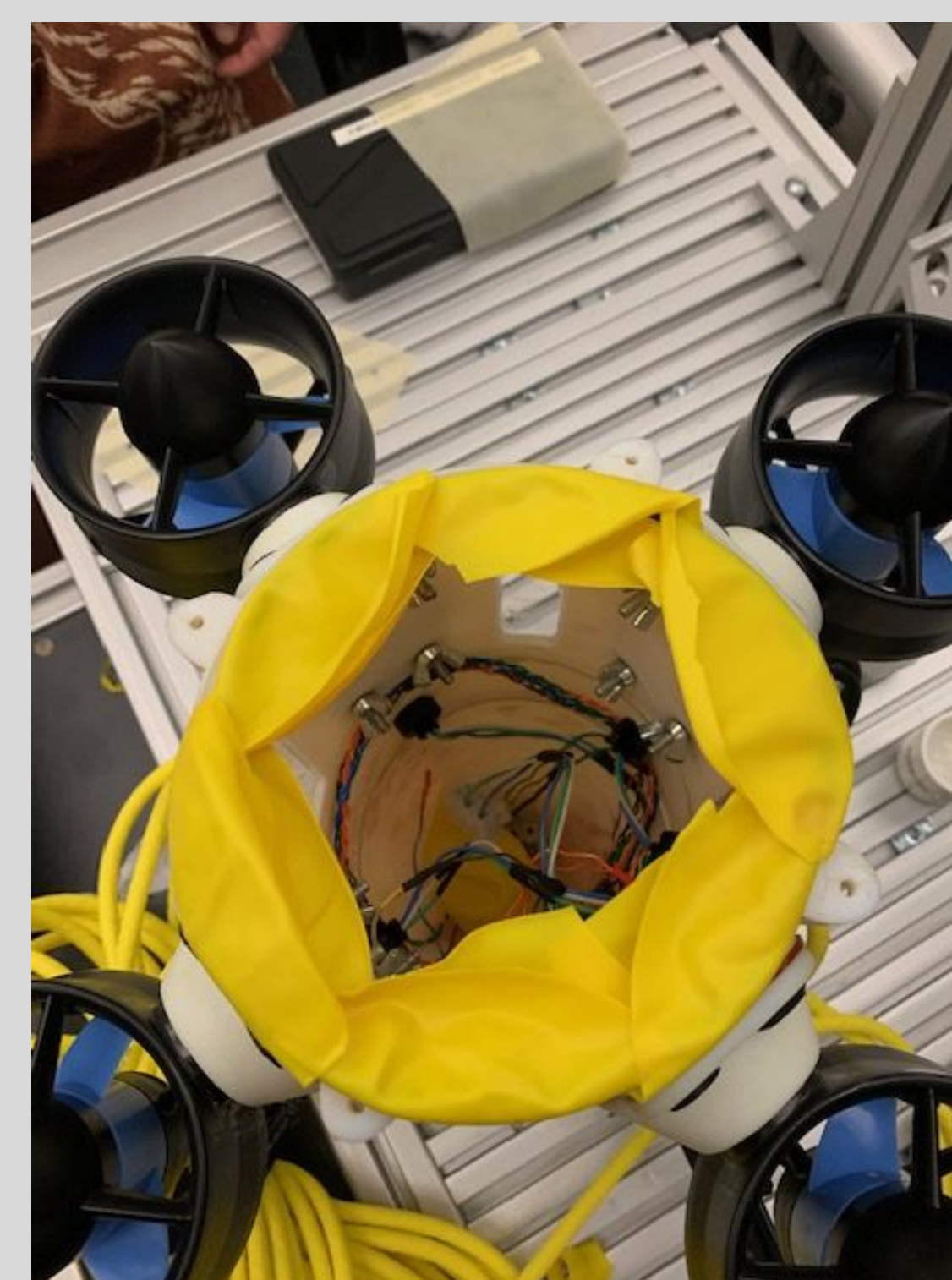
Figure 3: Balloons Seal to be tested for waterproofing
