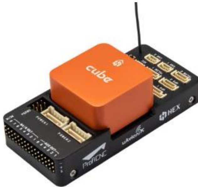
Fig. 3 Cube Orange that is the brain of the drone.
