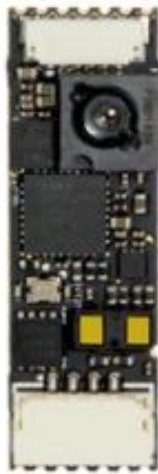
Fig. 6 Hereflow sensor to allow for indoor and more accurate outdoor flight.
