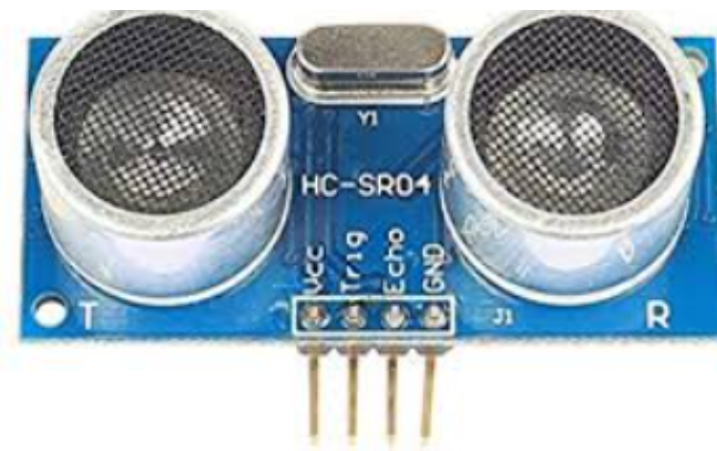
Fig. 4: Sonar rangefinder sensor to allow for indoor and more accurate outdoor flight.
