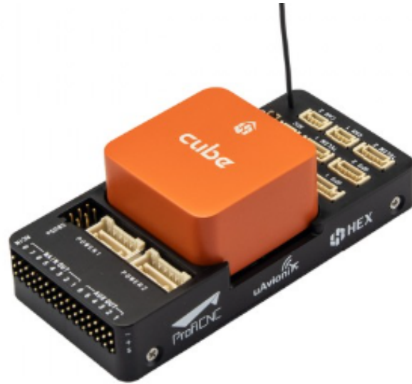
Fig. 3: The Cube Orange is the brain of the drone.
