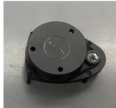
Fig. 7: Lidar360 that rotates in 360 degrees of motion to scan the terrain for object avoidance.
