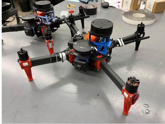
Fig. 29: Final drones in the lab ready to have the props attached for flight.
