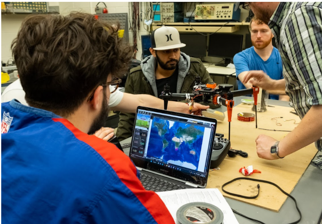
Fig. 26: Team programming initial drone with ArduPilot before the first test flight.
