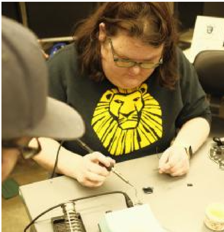
Fig. 21: Team member applying flux paste to her soldered board.
