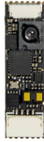
Fig. 6: The Here Flow which captures an image and uses radio waves to enable the drones to sense the height that they are flying at.
