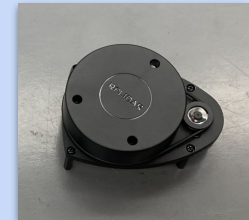
Slamtec Rplidar (Object avoidance sensor)
