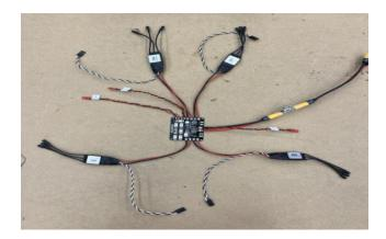
Fully soldered components. Long black components are to the motors and the long yellow wire is to the battery.
